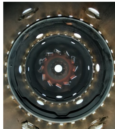
Fig. 15 Fire tube primary zone after testing
