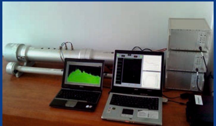
Studies and measurements for the determination of acoustic absorption coefficient and acoustic impedance of sound-absorbing materials with the Kundt tube set.
