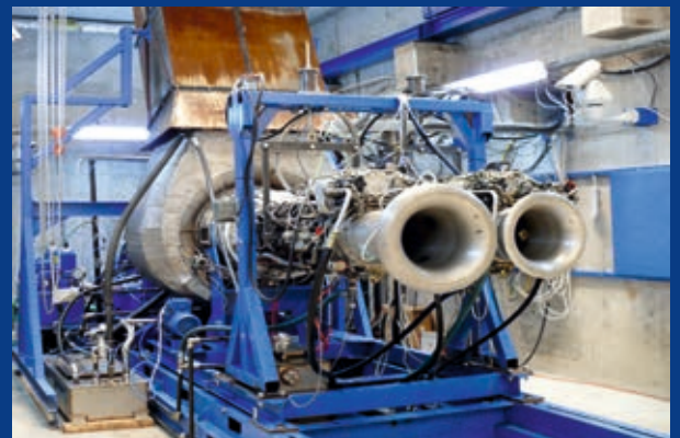
Twin engine TV-117A for industrial application
