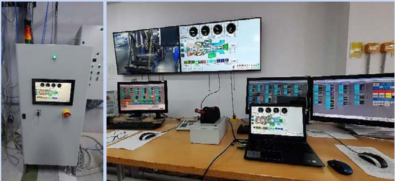
Automation system designed for testing ST40M marine gas turbine engines
