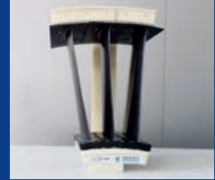
Triplet OGV mounted on a 3D printed stator case section
