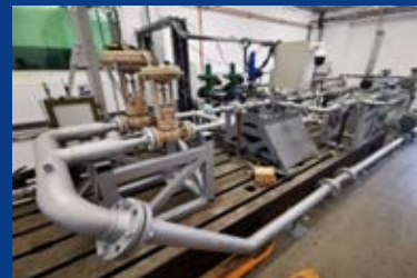
Test bench for pumps and turbo-pumps for launchers (similitude conditions water/N 2 , shaft power max. 600kW/10000rpm or 250kW/25000rpm, N 2 flow max. 5 kg/s)
