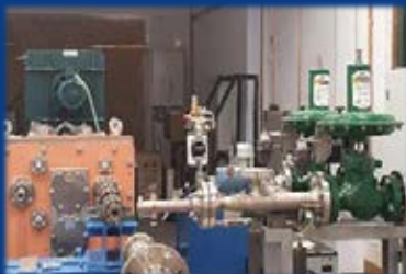
Test bench for pumps and turbo-pumps for launchers (similitude conditions water/N 2 , shaft power max. 600kW/10000rpm or 250kW/25000rpm, N 2 flow max. 5 kg/s)
