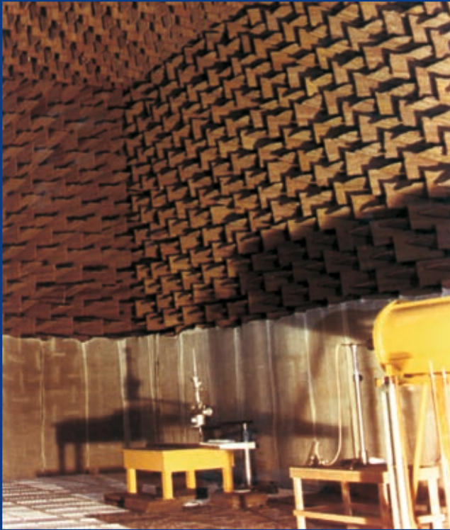
Acoustic tests - Anechoic chamber (1,200 m 3 ).
