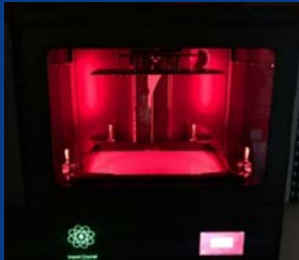
Liquid Crystal Magna 3D Printer Technology: DLP 3D printing Build volume: 510x280x350mm Printing speed: 13.3 mm/h (at 100 µm) Layer thickness: from 25 to 100 µm
