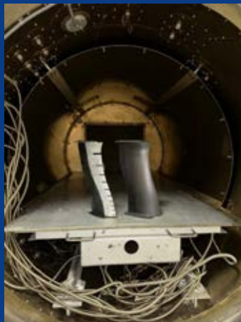
1/3 scale 3D printed OGV prototypes aero-acoustically tested
