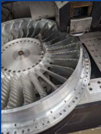
1/3 scale 3D printed OGV prototypes aero-acoustically tested
