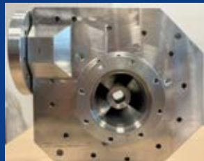
Electrically Driven Pump Feed Systems for 25kN LOX/LCH 4 Regeneratively Cooled Rocket Engines)
