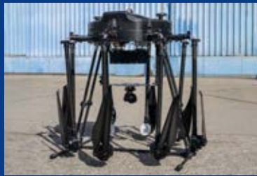
CFRP composite structure for Octocopter UAV equipped with hybrid propulsion solution
