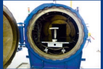
Autoclave - Scholz Ø1500 mm; length 2500 mm max. 400°C; max.20 bar; 6 vacuum lines/
