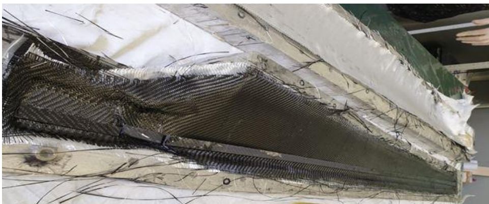
Figure 6. The insertion of the carbon rod.
