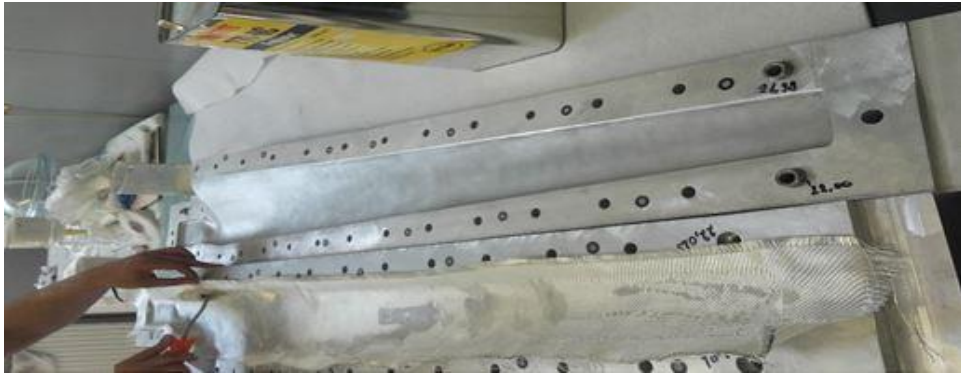
Figure 4. Disposing the first fiberglass layup.
