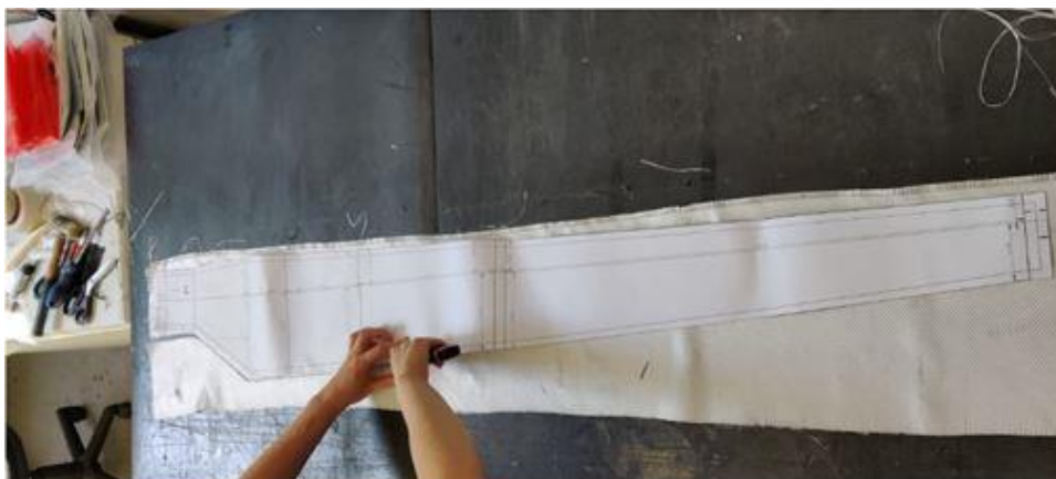
Figure 3. Cutting process of the layups.
