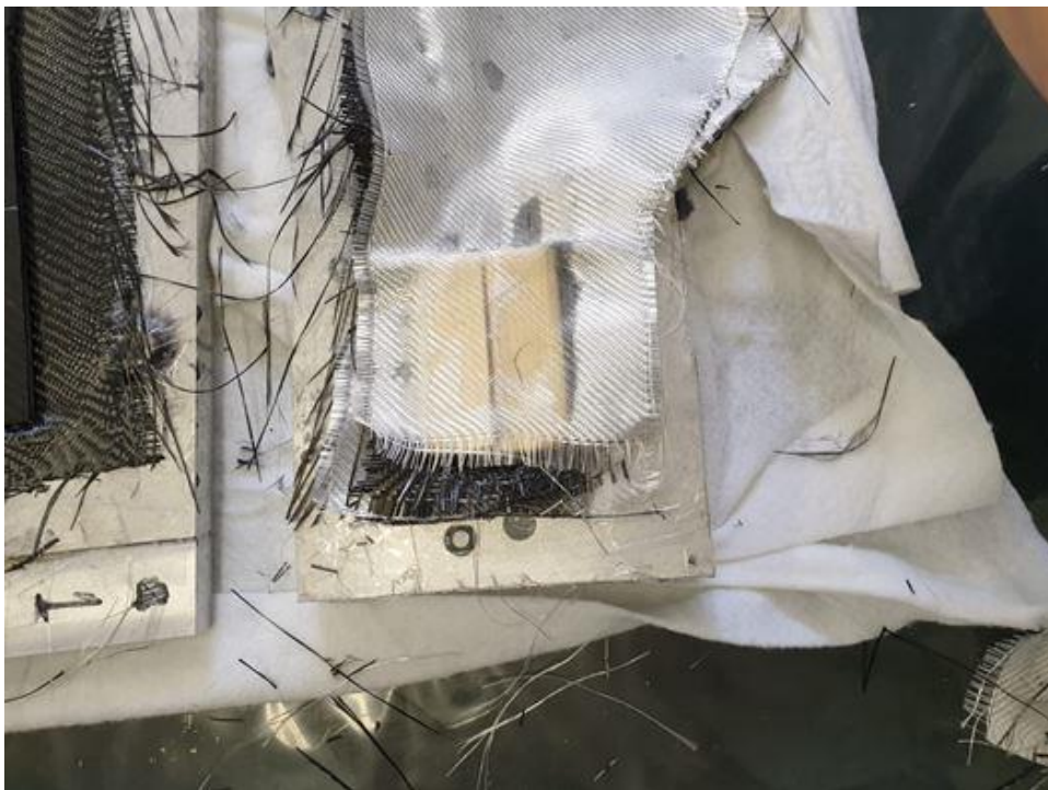
Figure 8. Fixed gripping area with the wooden structure.
