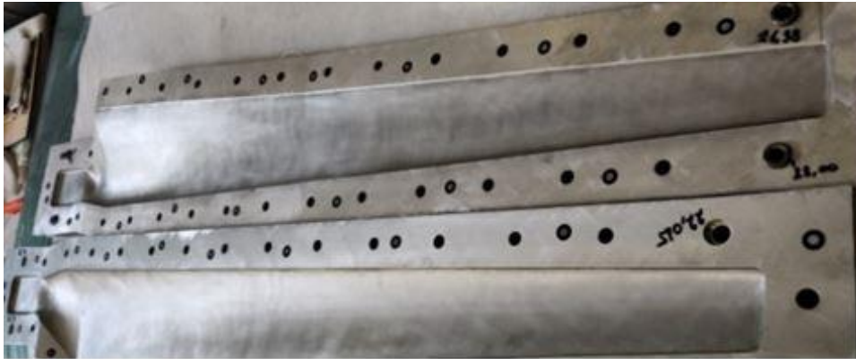
Figure 2. Moulds used for the manufacturing of the blades.
