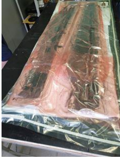
Figure 9. Vacuum bag sealing process.
