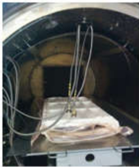
Figure 12. Vacuuming the mold
