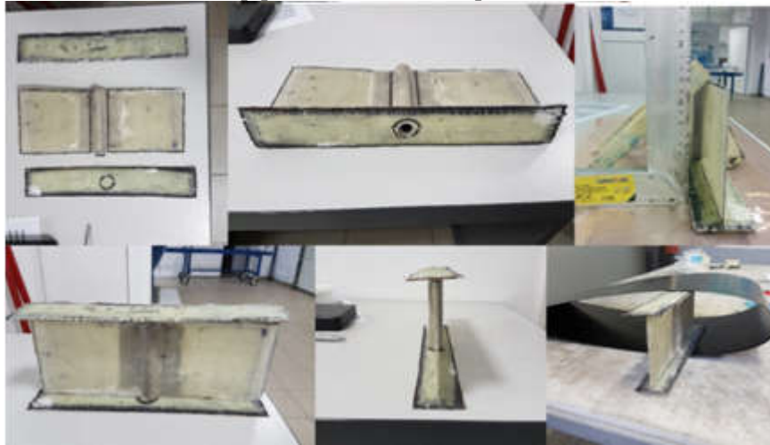
Figure 15. Joining the components that form the span section in the leading edge
