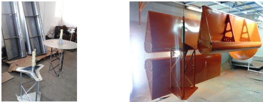
Figure 9. Blades and upper parts from the main pillar before and after the painting procedure.
