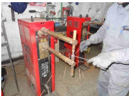
Figure 7. Pressure welding (left) and electric resistance welding (right).
