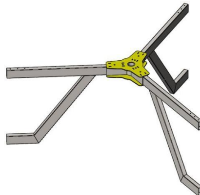
Figure 3. The arm system used for supporting the blades.
